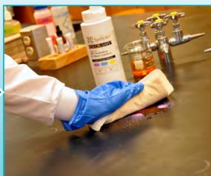
Use Hazmat Sorbents to clean up excess left from neutralization
